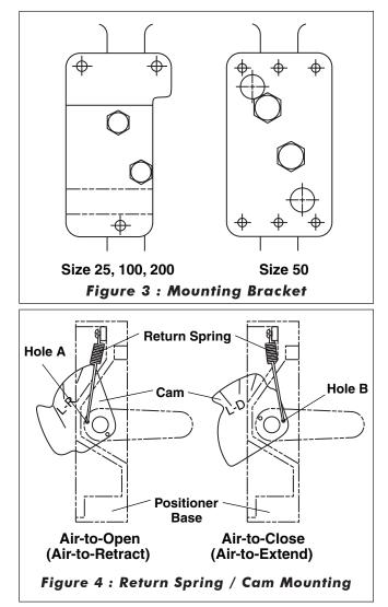
**Reversing Air Action on Linear Actuators**
