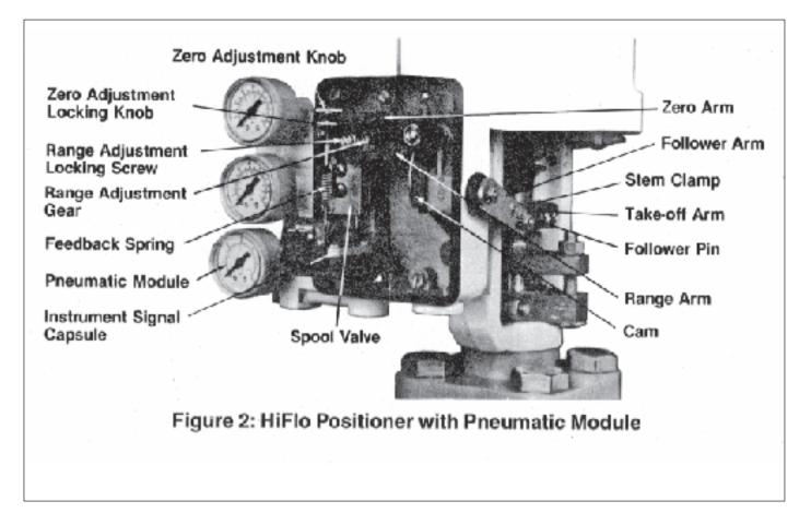
The downward motion of the balance beam leads to pulling of the pilot valve spool downward. The pilot valve ports open, and air is supplied to port 1 and exhausting air from port 2. The upward movement of the actuator piston occurs.
